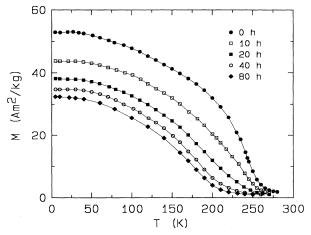
FIG. 4. Typical temperature dependence of the magnetization in an external field of 0.5 T of Mn<sub>1.5</sub>Sn after various periods of milling.
