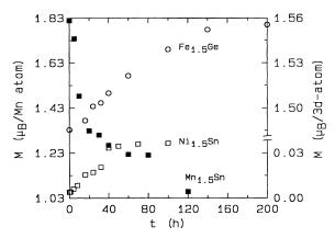
FIG. 3. Magnetization at 4.2 K of Mn<sub>1.5</sub>Sn (filled squares and the left-hand-side scale), Fe<sub>1.5</sub>Ge (open circles) as well as Ni<sub>1.5</sub>Sn (open squares and the right-hand-side scale) at 21 T as a function of milling time.
