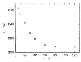
FIG. 5. Curie temperature  $(T_C)$  of  $Mn_{1.5}Sn$  as a function of milling time.
