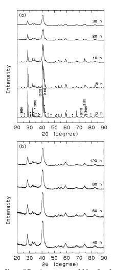
FIG. 1. X-ray-diffraction patterns of  $Mn_{1.5}Sn$  after various periods of milling.
