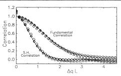
FIG. 3. Fundamental and second harmonic correlation in transmission as a function of sample rotation. Symbols are experimental data for  $\triangle$ ,  $L=27~\mu\mathrm{m}; \circ$ ,  $L=38~\mu\mathrm{m}; \diamondsuit$ ,  $L=65~\mu\mathrm{m}$ , with L the thickness of the sample. Smooth lines: theoretical curves.
