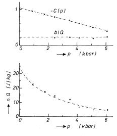
FIG. 4. The parameters C(p), b/Q, and nQ describing the anomalous part of the anisotropy energy of gadolinium at 4.2 K. Values for C(p) and nQ below 2 kbar have been calculated assuming a value for b/Q of 0.23, see text.
