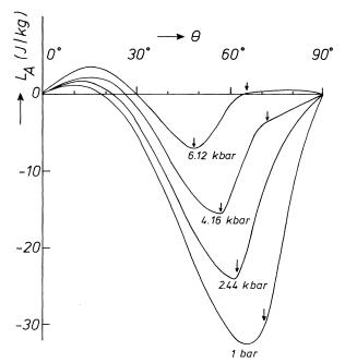
FIG. 1. The magnetic torque of gadolinium in the (c, a) plane at 4.2 K at different pressures. The edges of the "transition region" are marked by small arrows.
