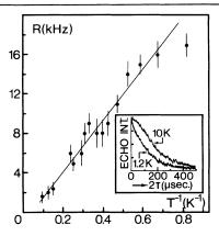
FIG. 3. Spin dephasing rate (R) of  $F^+$  centers vs  $T^{-1}$  between 1.2 and 10 K. Drawn line is best fit for  $R=2.6 \times 10^4 \ T^{-1}-1.1\times 10^3$  kHz. Inset shows optically detected spin-echo decays of  $F_2^{2+}$  center (microwave frequency is 1.870 GHz) at 1.2 and 10 K, respectively.
