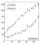
FIG. 2. Magnetic field dependence of C(z) (circles) and R (squares) when the  $F_2^{2+}$ -center spin-echo decay is fitted to the form  $\exp[-C(z)B(\tau)^{1/2}]$ , where  $B(\tau)$  is defined in the text. Drawn curves represent best fits, namely  $C(z) \propto z/(1+z^2)^{1/2}$  and  $R \propto H_z^2$ .
