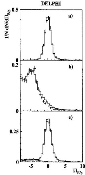
Fig. 2. Distribution of the pull on  $E/p$  for the electron hypothesis,  $\Pi_{E/p}$ , for a) an electron test sample, b) a hadron test sample and c) after all other electron identification cuts. The points with error bars are real data, the unshaded histogram is simulated data, and the shaded histogram is the simulated background from  $\tau$  decays. The discrepancy in the HPC response to hadrons is clearly visible.
