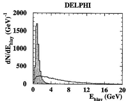
Fig. 3. Distribution of the average energy per layer  $E_{\text{hlay}}$  in the hadron calorimeter for real data test samples of pions (unshaded histogram) and of muons (shaded histogram). Entries with  $E_{\text{hlay}} = 0$  have been suppressed.
