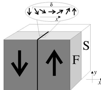
FIG. 1. The superconductor-ferromagnet junction. The domain wall.
