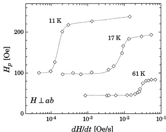
FIG. 1. For the specimen with an ellipsoidal-like cross section, the first flux penetration field  $H_p$  vs the applied magnetic field sweep rate  $dH/dt$  is displayed for different temperatures. The dotted lines are guides to the eyes. The data are scaled with the demagnetization factor  $N = 0.96 (\pm 15\%)$ .
