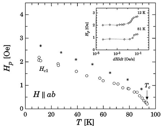
FIG. 4. Temperature dependence of  $H_p$  ( $H \parallel ab$ ) for a specimen with rectangular cross section and size  $2 \times 3.9 \times 0.05 \text{ mm}^3$  for different sweep rates: (\*)  $dH/dt \geq 6 \times 10^{-2} \text{ Oe/s}$  and (O)  $dH/dt \leq 6 \times 10^{-3} \text{ Oe/s}$ . The inset shows the  $H_p$  vs  $dH/dt$  dependence at  $T = 12$  and  $81 \text{ K}$ .
