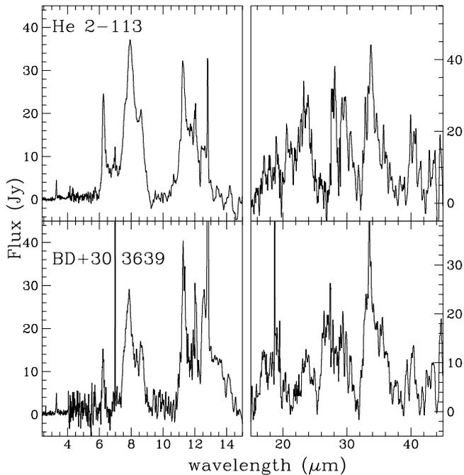
**Fig. 2.** Continuum subtracted 2.4–45  $\mu\text{m}$  spectra of He 2-113 (top) and BD+30 3639. Notice the prominent UIR emission bands at 3.3, 6.2, 7.7, 8.6, and 11.3  $\mu\text{m}$ , often attributed to Polycyclic Aromatic Hydrocarbons. At longer wavelengths emission from crystalline silicates is found (olivines, pyroxenes).
