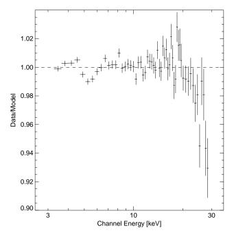
FIG. 8.—Ratio between the power-law fit of eq. (B1) and the PCA Crab nebula data. The major deviations between the data and the model are due to the Xe  $L_{1.2.3}$  edges at  $\sim 5.1$  keV and to the Xe K edge at 34.6 keV.
