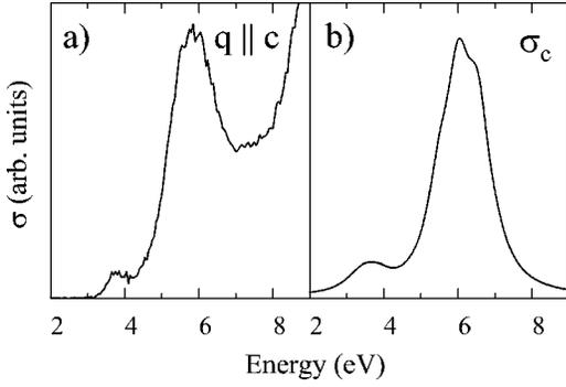
FIG. 6. The optical conductivity of  $\text{CuGeO}_3$  (a) derived from the experimental loss function with  $\mathbf{q} \parallel \mathbf{c}$  using the Kramers-Kronig relations and (b) calculated within the  $\text{Cu}_5\text{O}_{12}$  cluster model.
