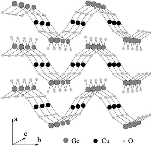
FIG. 1. Crystal structure of  $\text{CuGeO}_3$ . Copper atoms are shown as black spheres, oxygen atoms as light grey spheres, and germanium atoms as dark grey spheres.
