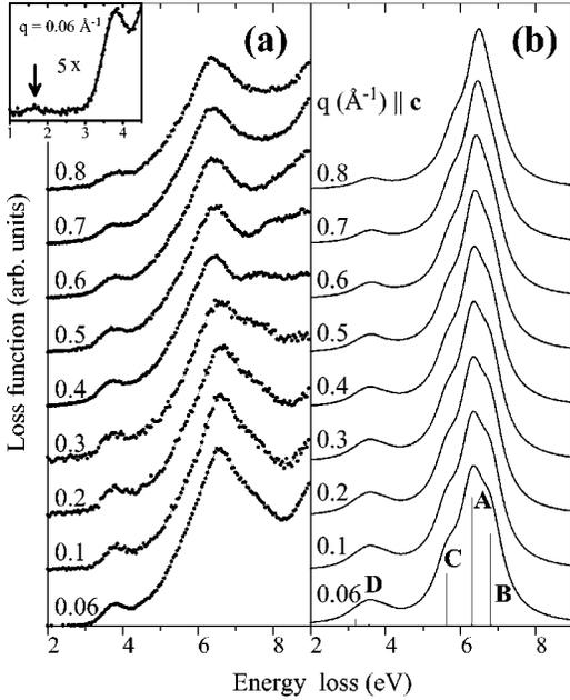
FIG. 3. The loss functions of  $\text{CuGeO}_3$  (a) measured using EELS in transmission with momentum transfer aligned along the crystallographic  $c$  direction and (b) calculated using a one-dimensional extended multiband Hubbard model at half filling. The inset shows the fivefold magnified experimental spectrum below 4.5 eV measured with  $q=0.06 \text{ \AA}^{-1}$ .
