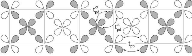
FIG. 2. Cu<sub>5</sub>O<sub>12</sub> cluster used in the calculations of the loss functions and the optical conductivity of CuGeO<sub>3</sub>. In the model only the Cu  $3d_{x^2-y^2}$  and O  $2p_{x(y)}$  orbitals are taken into account. The cluster is divided into two sublattices each marked by either shaded or unshaded orbitals. The definition of the hopping amplitudes  $t_{pd}^\sigma$ ,  $t_{pd}^\pi$  and  $t_{pp}$  is symbolically given by the double arrows. See text for details.
