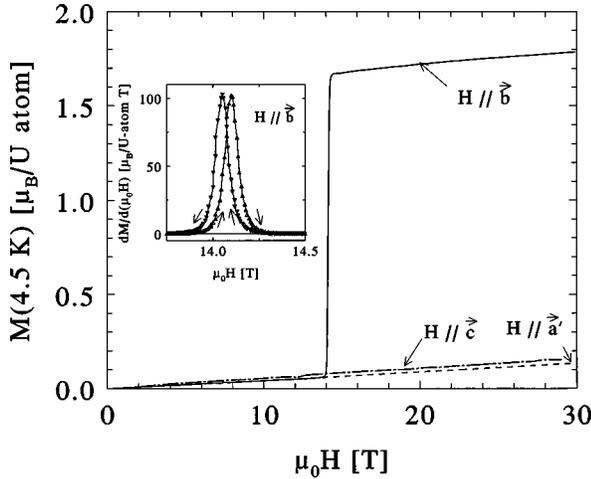
FIG. 2. Magnetization,  $M_i(H)$ , vs pulsed magnetic field ( $\vec{H} \parallel \vec{a}'$ , dashed line;  $\vec{H} \parallel \vec{b}$ , solid line; and  $\vec{H} \parallel \vec{c}$ , dash-dotted line). The inset shows the field derivative  $dM_b/d(\mu_0 H)$  close to the metamagnetic transition (field sweep up,  $\triangle$  and field sweep down,  $\nabla$ ).
