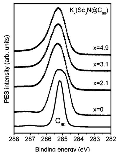
FIG. 5. X-ray photoemission spectra of  $K_x(Sc_3N@C_{80})$  at the  $C 1s$  core level as a function of increasing  $K$  intercalation. The  $C 1s$  spectrum of  $C_{60}$  (gray) is shown for comparison.
