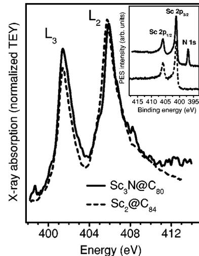
FIG. 1. X-ray absorption spectra of  $\text{Sc}_3\text{N}@C_{80}$  and  $\text{Sc}_2@C_{84}$  at the Sc  $L_{2,3}$  edge. Inset: photoemission spectra of the same materials (solid line:  $\text{Sc}_3\text{N}@C_{80}$ ; dashed line:  $\text{Sc}_2@C_{84}$ ) in the binding energy range covering the Sc  $2p$  and N  $1s$  core levels.
