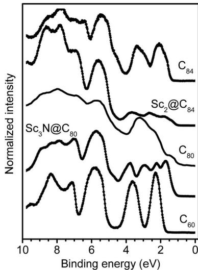
FIG. 3. Valence band photoemission spectra of the metallofullerenes  $\text{Sc}_3\text{N}@C_{80}$  and  $\text{Sc}_2@C_{84}$ , with the analogous spectra of the “empty” fullerenes  $C_{60}$ ,  $C_{80}$ , and  $C_{84}$  shown for comparison. The spectrum of  $C_{80}$  is taken from Ref. 12.
