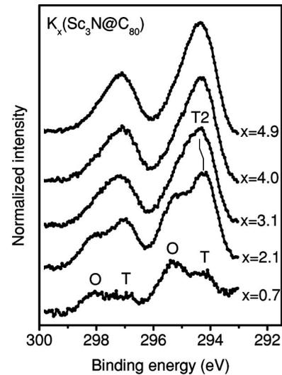
FIG. 4.  $K 2p$  core level photoemission spectra for the system  $\text{K}_x(\text{Sc}_3\text{N}@C_{80})$  as a function of increasing K intercalation level,  $x$ . The labels T and O refer to signal originating from K ions situated in interstitial sites of a tetrahedral or octahedral type, respectively.
