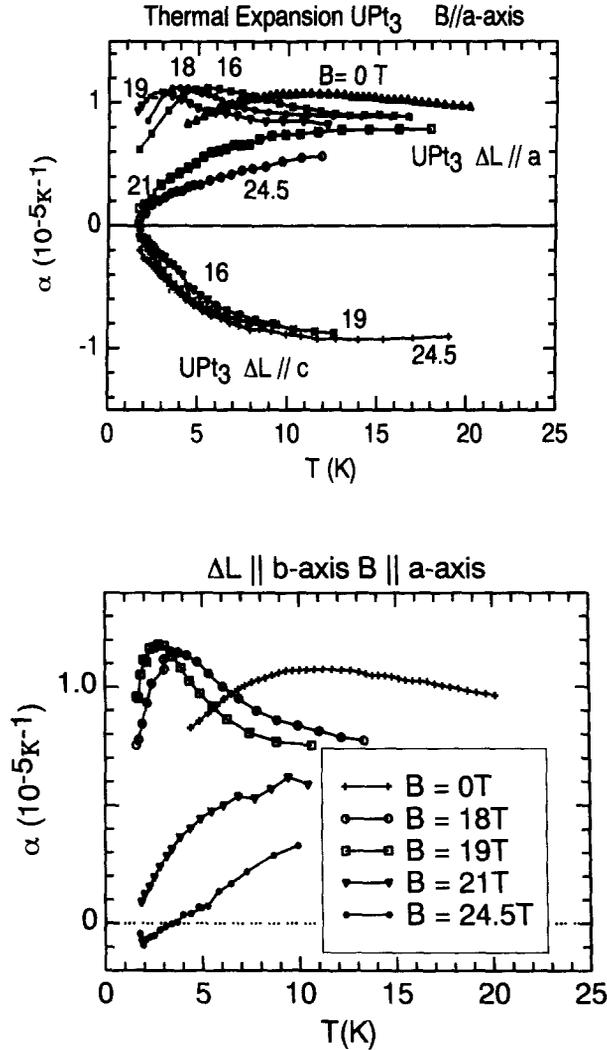
Fig. 1. Thermal expansion data of  $UPt_3$  along the three main crystallographic directions for the applied field parallel to the  $a$ -axis in the hexagonal plane and for field values below and above the meta-magnetic field of 20 T [11].
