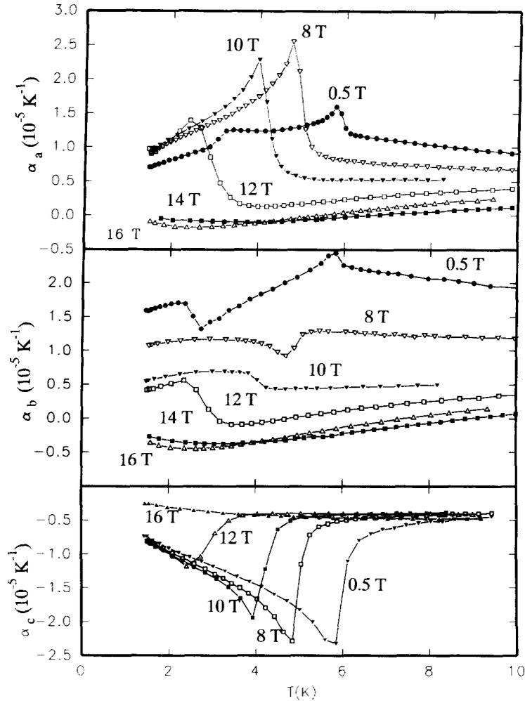
Fig. 2. Thermal expansion data of  $U(Pt_{0.95}Pd_{0.05})_3$  along the three main crystallographic directions for the applied field parallel to the  $a$ -axis in the hexagonal plane and for field values below and above the meta-magnetic field of approximately 12 T [11].
