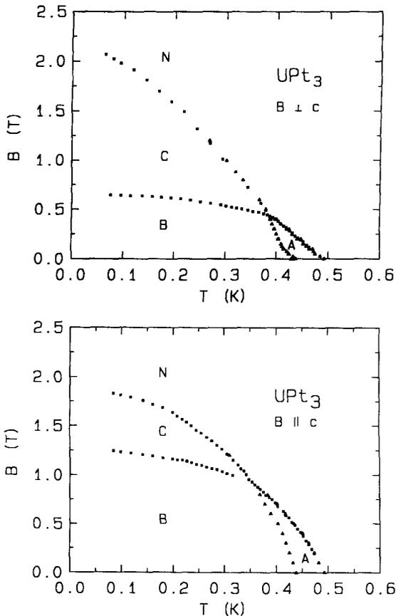
Fig. 6. The superconducting phase diagram of  $\text{UPt}_3$  for fields applied perpendicular and parallel to the hexagonal axis, as studied by thermal expansion and forced magnetostriction measurements [6].
