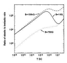
FIG. 4. Temperature dependence of the ratio of elastic to inelastic rate constant ( $\alpha_{\rm el}/\alpha_{\rm in}$ ), in fields B=10 G, B=750 G, and B=100 kG.
