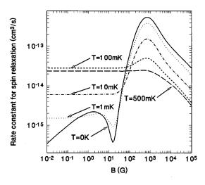
FIG. 1. Rate constant for spin relaxation ( $\alpha_{rel}$ ) as a function of B for several values of T (0, 1, 10, 100, and 500 mK).
