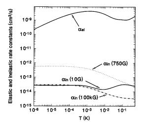
FIG. 3. Rate constants of elastic ( $\alpha_{\rm el}$ ) and inelastic ( $\alpha_{\rm in}$ ) collisions as functions of T. The upper curve corresponds to  $\alpha_{\rm el}$ , and the three lower curves to  $\alpha_{\rm in}$  in fields B=10 G, B=750 G, and B=100 kG.
