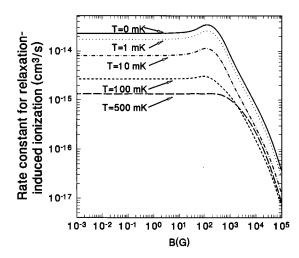
FIG. 2. Rate constant for relaxation-induced ionization ( $\alpha_{ri}$ ) as a function of *B* for several values of *T* (0, 1, 10, 100, and 500 mK).
