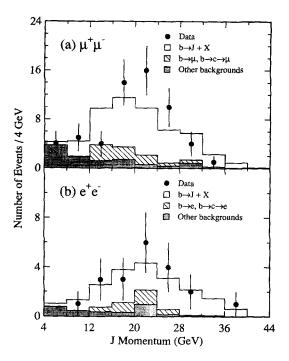
Fig. 4. The J momentum distributions from (a) the  $\mu^+\mu^-$ , and (b) the e<sup>+</sup>e<sup>-</sup> channels. The fit result and the background contributions are also shown.
