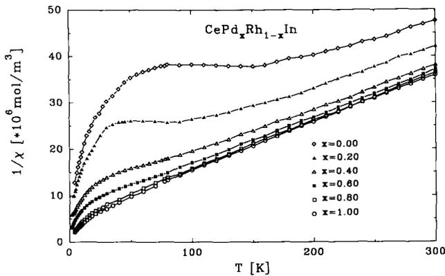
Fig. 4. Dependence on temperature of the inverse magnetic susceptibility of some  $\text{CePd}_x\text{Rh}_{1-x}\text{In}$  compounds. The lines are guides to the eye.
