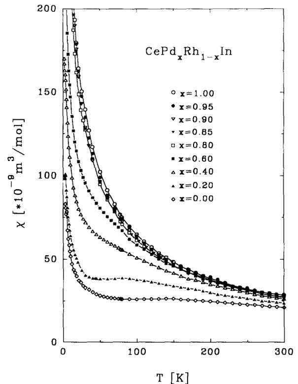
Fig. 3. Dependence on temperature of the magnetic susceptibility of  $\text{CePd}_x\text{Rh}_{1-x}\text{In}$ . The lines are guides to the eye.
