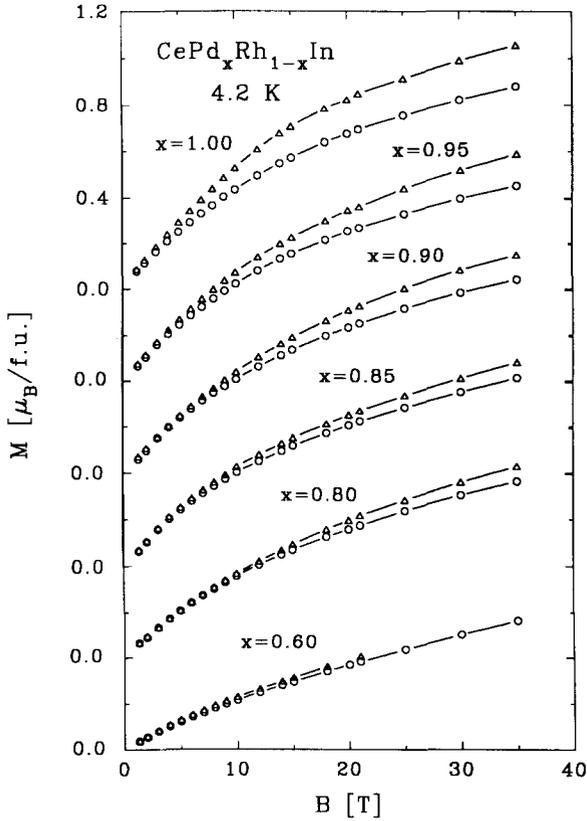
Fig. 6. Development of anisotropy in the field dependence of the magnetization with increasing Pd content in  $\text{CePd}_x\text{Rh}_{1-x}\text{In}$ . The triangles represent measurements on powder free to be oriented in the field, whereas the circles represent results obtained on powder fixed in random orientation by frozen alcohol.
