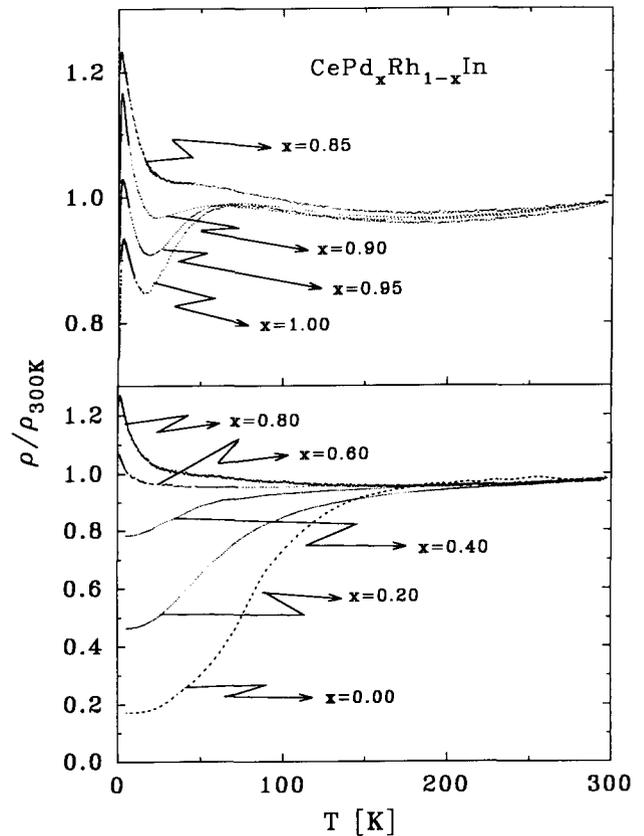
Fig. 9. Dependence on temperature of the electrical resistivity of  $\text{CePd}_x\text{Rh}_{1-x}\text{In}$  normalized to the room temperature value. The result for pure  $\text{CeRhIn}$  (dashed curve) is taken from ref. 5.
