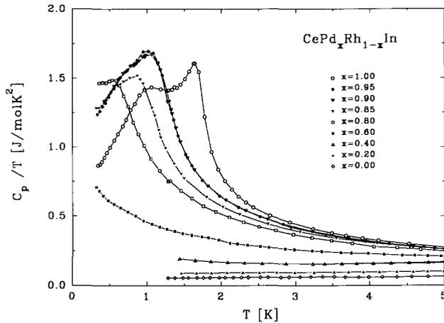
Fig. 8. Low-temperature part of the temperature dependence of the specific heat of  $\text{CePd}_x\text{Rh}_{1-x}\text{In}$  for  $x \geq 0.6$  in the representation  $C_p/T$  vs.  $T$ . The lines are guides to the eye.
