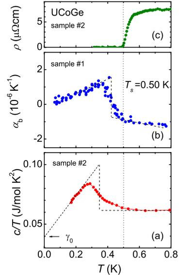
FIG. 3. (Color online) (a) Specific heat of UCoGe (single crystal #2) in a plot of  $c/T$  versus  $T$ . (b)  $\alpha_b(T)$  of UCoGe (single crystal #1). (c) Resistivity versus  $T$  of UCoGe (single crystal #2). The vertical dotted line indicates the approach to the zero-resistance state coinciding with the onset temperature of bulk SC as seen in  $c/T$  and  $\alpha_b(T)$ . The dashed lines in (a) and (b) represent idealized sharp FM and SC transitions.
