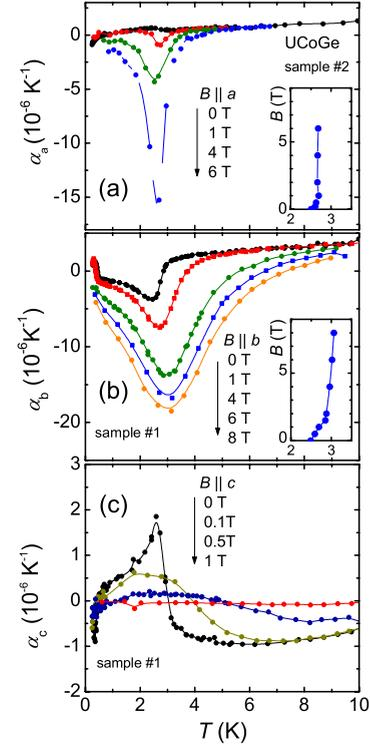
FIG. 5. (Color online) Coefficient of thermal expansion of UCoGe in applied magnetic fields along the dilatation direction as indicated. (a)  $\alpha_a$  for  $B \parallel a$ ; (b)  $\alpha_b$  for  $B \parallel b$ ; and (c)  $\alpha_c$  for  $B \parallel c$ . Insets:  $T_c$  as a function of  $B \parallel a, b$ .
