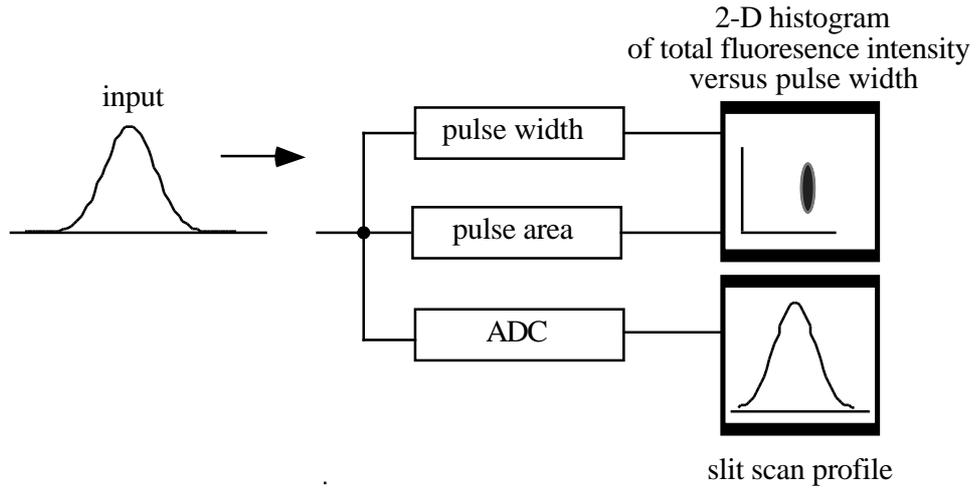
FIGURE 2: Modes of operation of the data acquisition equipment. In the experiments described in this paper the 2-dimensional histogram is measured and further analyzed to obtain an average pulse width. The pulse area box measures the total (integrated) fluorescence intensity; the ADC box measures pulse profiles and the pulse width box measures the width of the fluorescence pulse.
