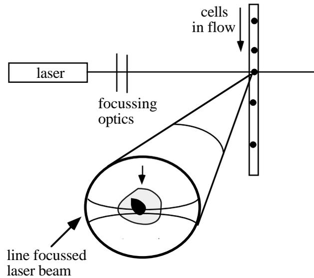
FIGURE 1: A schematic drawing of the slit scan principle. Hydrofocussed cells in a flow pass the line focussed laser beam one by one. The stained nucleus produces a fluorescence signal. The width of the fluorescence pulse is a measure of the nuclear diameter.
