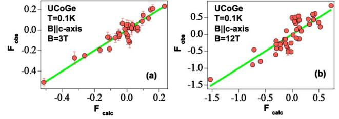
FIG. 2. (Color online) Observed versus calculated (solid line) magnetic structure factor of UCoGe for the polarized neutron-diffraction experiment at  $T = 0.1$  K in an applied field ( $B\parallel c$ ) of (a) 3 T and (b) 12 T.
