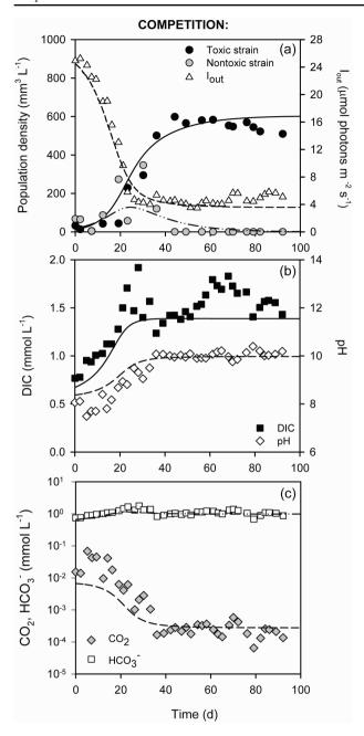
Figure 6.3. Competition between the toxic strain *Microcystis* CYA140 and nontoxic strain *Microcystis* CYA43 in a  $CO_2$ -limited chemostat. (a) Population densities of the competing strains (expressed as biovolumes) and light intensity penetrating through the chemostat ( $I_{out}$ ), (b) dissolved inorganic carbon (DIC) and pH, and (c)  $CO_2$  and bicarbonate concentrations. Symbols represent chemostat data, lines show the model predictions. Parameter values are provided in Appendix 3.
