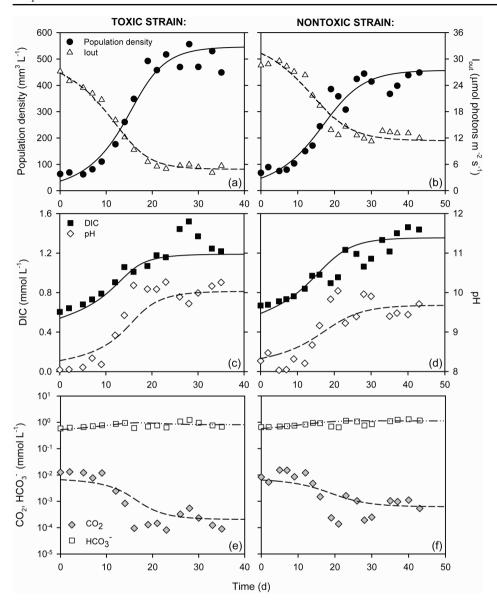
Figure 6.1. Monoculture experiments of the toxic strain Microcystis CYA140 and nontoxic strain Microcystis CYA43 in CO<sub>2</sub>-limited chemostats. (a, b) Population density (expressed as biovolume) and light intensity penetrating through the chemostat ( $I_{out}$ ), (c, d) dissolved inorganic carbon (DIC) and pH, and (e, f) CO<sub>2</sub> and bicarbonate concentrations. Symbols represent chemostat data, lines show the model fits. Parameter values are provided in Appendix 3.
