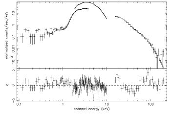
**Fig. 5.** Data and best fit model for the broad band BeppoSAX spectrum of interval E. Count-rates from all the three instruments (LECS, MECS and PDS) are shown here together with their residuals with respect to the model (in units of individual contributions to the  $\chi^2$ )
