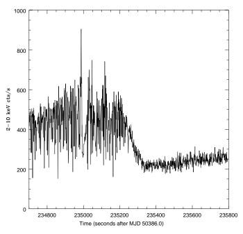
**Fig. 3.** Zoom-in (bin size 1 s) of the MECS light curve of the outburst reported in Fig. 2, showing the complex timing behaviour of the source during the time intervals B and C. For this figure it looks very likely that the high frequency oscillations started earlier than the beginning of interval B, during the Earth occultation
