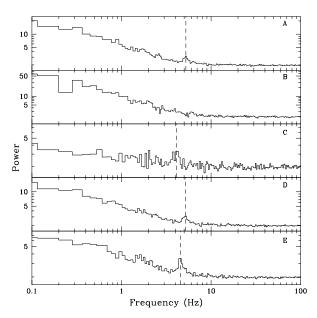
**Fig. 6.** Power Spectral Density obtained by the MECS data for the five intervals given in Fig. 2. Frequency bins are spaced according to a geometric series. The vertical dashed lines indicate the centroid of the QPO frequency at 5.23 Hz (A), 4.12 Hz (C), 5.16 Hz (D) and 4.58 Hz (E).
