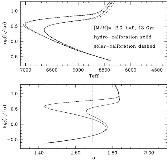
FIG. 1.—*Top*: Isochrones in the  $T_{\text{eff}}\text{-log}(L/L_{\odot})$  diagram for  $[M/H] = -2.0$ . Two isochrones ( $t = 9, 13$  Gyr) computed with  $\alpha_{\text{eff}}$  (solid lines) are compared to the corresponding isochrones computed with a constant  $\alpha_{\odot}$  (dashed lines). *Bottom*: Values of  $\alpha_{\text{eff}}$  along the hydrodynamic calibrated isochrones; the vertical line represents the constant  $\alpha_{\odot}$  of the standard isochrones.
