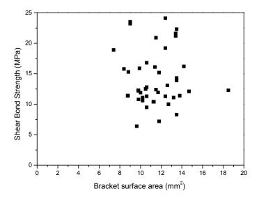
Figure 2.2 Shear bond strength (MPa) plotted against the bracket surface area (mm<sup>2</sup>). Linear regression showed that there was no correlation between the two variables ( $r^2 = 0.0$ ).
