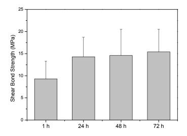
Figure 2.1 Shear bond strength (MPa) plotted against the debonding time. One-way ANOVA (F = 5.9; P = 0.001) showed significant difference between  $\frac{1}{2}$  -1 h and 24 h, 48 h, and 72 h.
