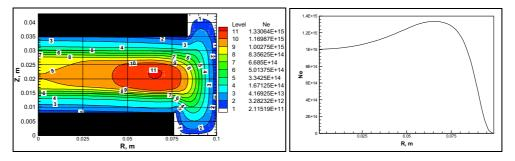
Fig. 4.3. Left: Spatial distribution of the electron concentration. R=0 corresponds to the axis of symmetry. Ne is the number of electrons per m3. Black plates denote electrodes. Right: electron concentration in the horizontal slice at Z=0.021 m (in the middle between the electrodes).
