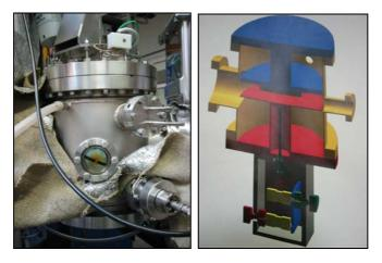
Fig. 4.1. Photo and engineering drawing of the ASTER reactor. The reactor gas chamber has the inner diameter of 200 mm and the height of 280 mm.
