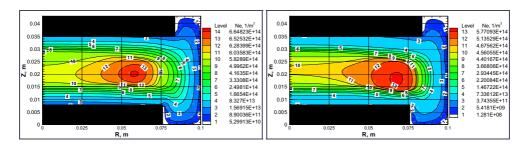
Fig. 4.4. Spatial distribution of electron concentration averaged over RF cycle for different pressures.
