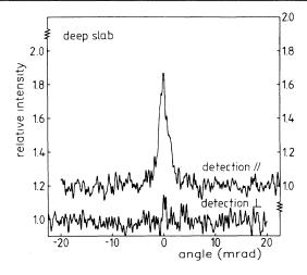
FIG. 3. Parallel and perpendicularly polarized difference in critical backscattering from the slab between 70 and 1500  $\mu$ m of 9.6 vol% of 1.091- $\mu$ m polystyrene in water. Upper curve: detected light polarized parallel to incident light. Lower curve: detected light polarized perpendicular to incident light.
