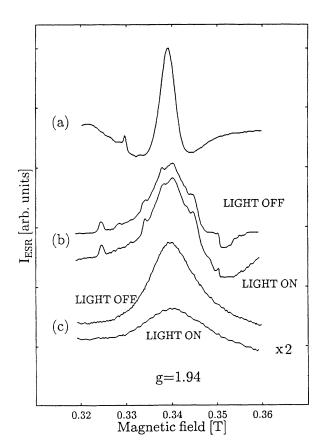
FIG. 1. Electron-spin-resonance spectra of LPE-grown x=0.42 (a) and x=0.5 (b)  $\mathrm{Al}_x\mathrm{Ga}_{1-x}\mathrm{As}$  layers. The spectra shown in (b) were measured before and after the illumination. The ESR spectrum shown in (c) was measured for x=0.41 LPEE layer after removing the GaAs substrate. The ESR signal shown was observed for sample cooled down to 4 K temperature in total darkness before and after 120 s of white-light illumination.
