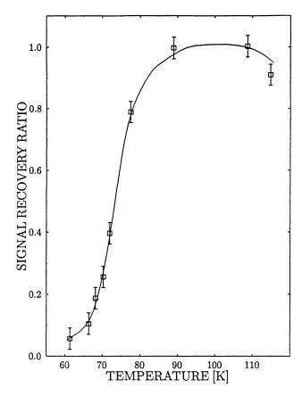
FIG. 3. Temperature dependence of the ESR signal recovery measured for the  $x = 0.41 \text{ Al}_x \text{Ga}_{1-x} \text{As LPEE}$  epilayer. The sequence of steps of the experiment is described in the text.
