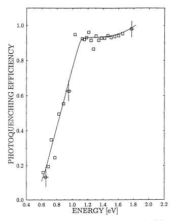
FIG. 2. Spectral dependence of the g=1.94 ESR signal photoquenching observed for the x=0.41 Al<sub>x</sub>Ga<sub>1-x</sub>As LPEE epilayer under illumination. The sequence of steps of the experiment is described in the text. 1 stands for total photoquenching of the signal.
