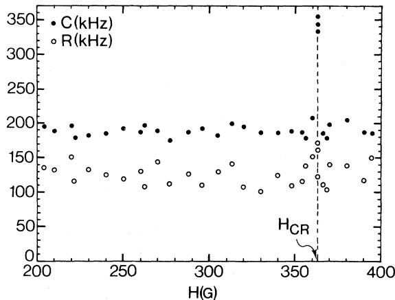
FIG. 2. Magnetic field dependence of  $C(z)$  ( $\bullet$ ) and  $R$  ( $\circ$ ) as obtained from fitting the  $F_2^{2+}$ -center echo decay curves to the form  $\exp[-C(z)B(\tau)^{1/2}]$ , as explained in the text. The sharp rise for  $H = 363$  G in  $C(z)$  is representative of CR between  $F_2^{2+}$  and  $F^+$  centers.
