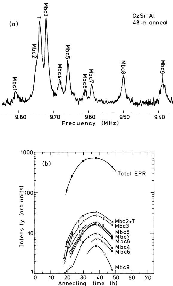
FIG. 2. FSENDOR results for the Al-doped Czochralski-grown silicon sample following annealing at  $470^\circ\text{C}$  for 48 h: (a) ENDOR spectrum with individual resonance lines corresponding to different species; (b) intensity of the overall EPR line and individual components corresponding to different species.
