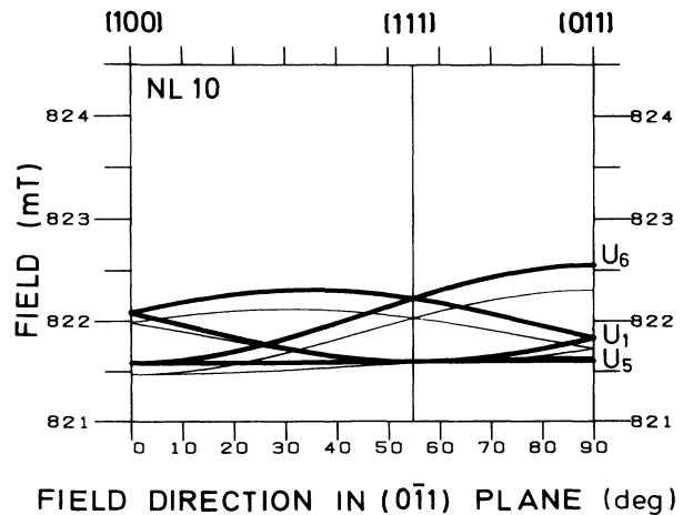
FIG. 1. Time dependence of the Si-NL10 EPR spectrum, or *g*-value shifting effect (23 GHz). The thick and thin lines correspond to 470°C annealing of 10 and 100 h, respectively. The  $U_1$ ,  $U_5$ , and  $U_6$  high-symmetry points are marked.
