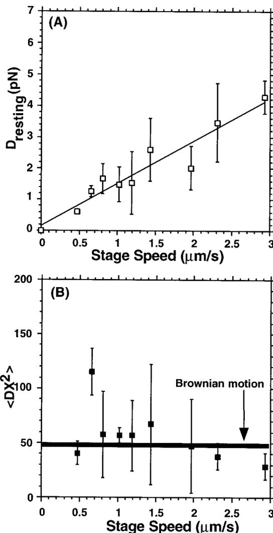
FIGURE 4 Plot of  $D_{\text{resting}}$  (A) and  $\langle DX^2 \rangle$  (B) against piezoelectric stage speed. Scanning was performed using a  $0.73\text{-}\mu\text{m}$  Qa-2 antibody-coated bead at  $37^\circ\text{C}$ . For each scan speed, eight beads were analyzed (error bars represent standard error of the mean).
