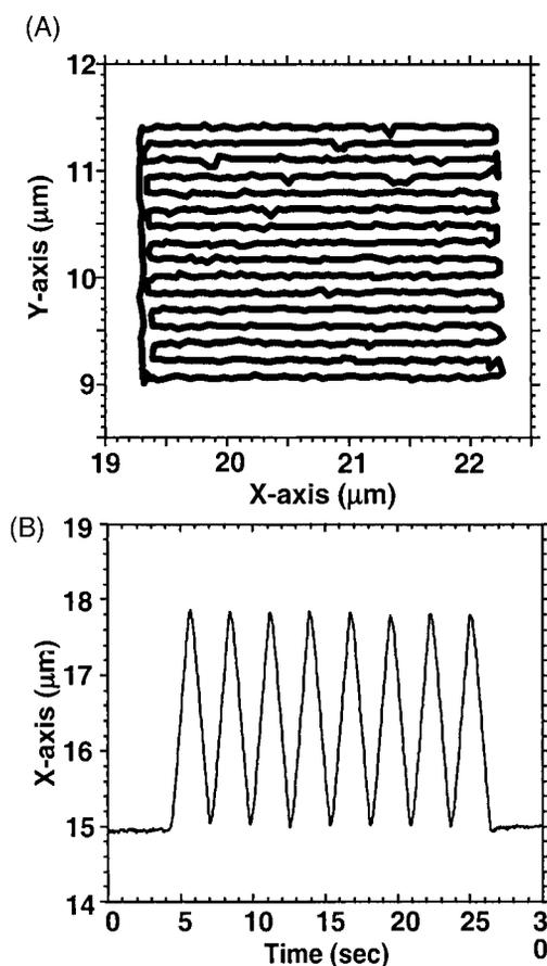
FIGURE 1 (A) Example of the scanning track of a 0.73- $\mu\text{m}$  bead attached to the coverslip. (B) Example of the relationship between time and the piezostage movement. The piezoelectric stage position was regulated by a computer, using a 2-D scanning program. Bead position was determined by the single-particle tracking (SPT) method (Gelles et al., 1988).
