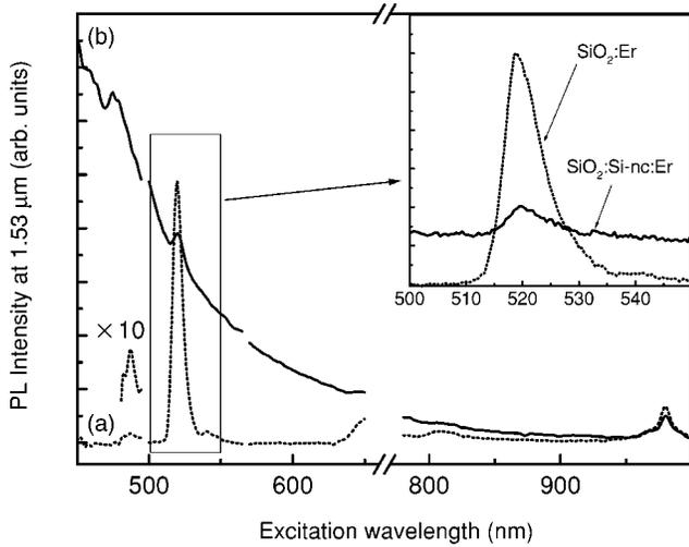
FIG. 1. Room-temperature photoluminescence excitation spectra for Sample No. 1 ( $\text{SiO}_2:\text{Er}$ ) (a) and Sample No. 2 ( $\text{SiO}_2:\text{Si-nc,Er}$ ) (b). Inset presents details of PLE spectra at  $\lambda_{\text{exc}} \approx 520$  nm, measured with maximum OPO power ( $\Phi \approx 3 \times 10^{25} \text{ cm}^{-2} \text{ s}^{-1}$ ).
