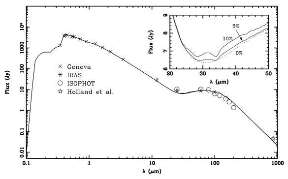
**Fig. 2.** Model infrared spectra for Vega. The parameters for the model are given in the text. The IRAS data are taken from Walker & Wolstencroft (1988), the ISOPHOT data are from Heinrichsen et al. (1998) and the submm flux is taken from Holland et al. (1998). The labels with the curves in the inset are the abundances of forsterite for the different models.
