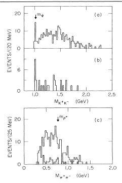
FIG. 1.  $K^+K^-$  mass distribution for (a) untagged and (b) tagged  $\gamma\gamma \to K^+K^-\pi^+\pi^-$  events. (c)  $\pi^+\pi^-$  masses for events without  $\phi$  mesons, i.e.,  $M(K^+K^-) > 1.04$  GeV, and (shaded) events with  $\phi$  mesons, i.e.,  $M(K^+K^-) < 1.04$  GeV; both tagged and untagged events included.
