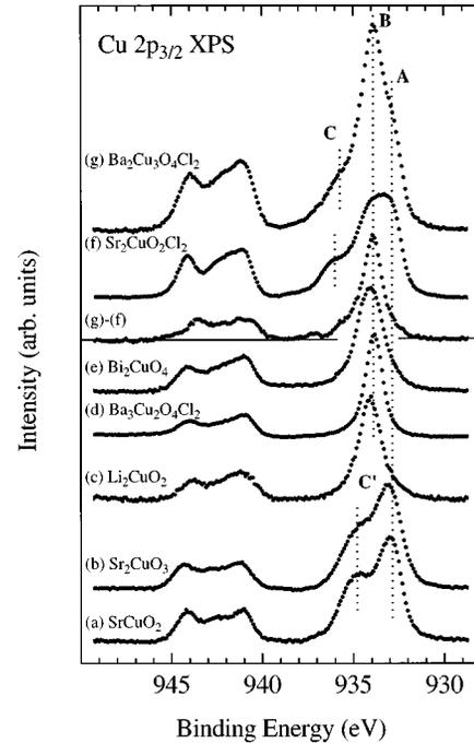
FIG. 2. Cu 2p<sub>3/2</sub> photoemission spectra of the single-crystalline cuprates. The 1D chain systems (a)  $\text{SrCuO}_2$ , (b)  $\text{Sr}_2\text{CuO}_3$ , (c)  $\text{Li}_2\text{CuO}_2$ , (d)  $\text{Ba}_3\text{Cu}_2\text{O}_4\text{Cl}_2$ , (e) 0D  $\text{Bi}_2\text{CuO}_4$ , and planar (f)  $\text{Sr}_2\text{CuO}_2\text{Cl}_2$  and (g)  $\text{Ba}_2\text{Cu}_3\text{O}_4\text{Cl}_2$ . Also shown is the difference spectrum (g)–(f).
