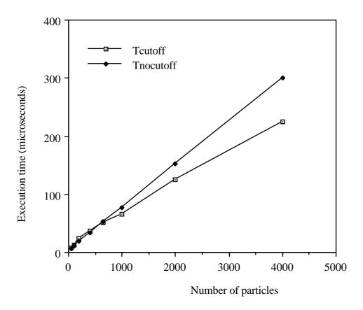
Fig. 3) The execution times for the vector implementation on the CRAY for the one particle potential energy loop both with potential cut-off and without potential cut-off.
