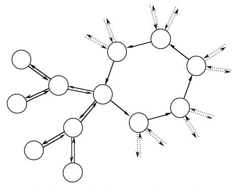
Figure 2) Diagram of hybrid implementation. Ring processors perform the annealing process, tree-slave processors perform energy function calculations, 7 in our implementation.
