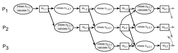
Figure 1) Diagram of a 3 processor implementation of the overlap algorithm.
