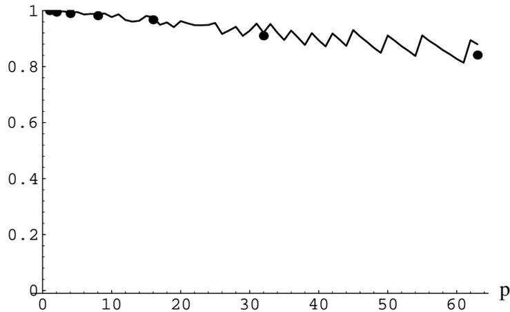
Figure 11: The efficiency on one iteration of the parallel PCGMR for  $n = 495$ , as a function of the number of processors. The black dots are the experimental results, the solid line is the theoretical efficiency.
