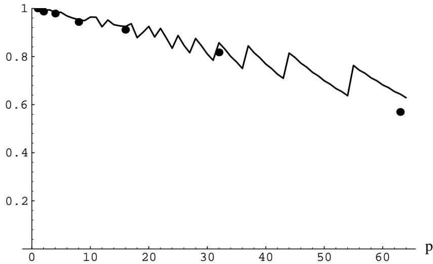
Figure 10: The efficiency on one iteration of the parallel PCGMR for  $n = 219$ , as a function of the number of processors. The black dots are the experimental results, the solid line is the theoretical efficiency.
