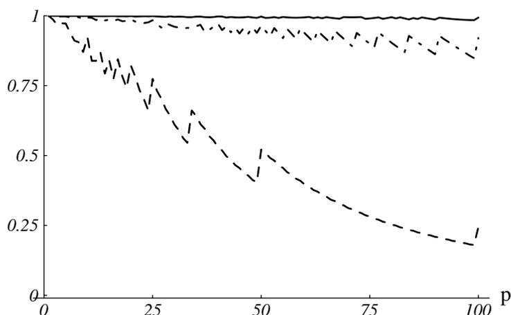
Figure 6: The theoretical efficiency for parallel PCGMR,  $m=0$ , with a rowblock decomposition of the matrix, implemented on a bidirectional ring of transputers. The dashed line is for  $n=100$ , the dot-dashed line is for  $n=1000$  and the full line is for  $n=10000$ ;  $p$  is the number of transputers
