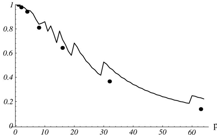
Figure 9: The efficiency on one iteration of the parallel PCGMR for  $n = 60$ , as a function of the number of processors. The black dots are the experimental results, the solid line is the theoretical efficiency.
