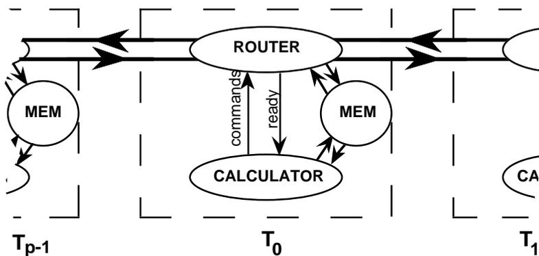
Figure 8: Main processes and streams in a transputer; MEM is the local memory, Router and Calculator are two OCCAM processes, and  $T_{p-1}$ ,  $T_0$ , and  $T_1$  are three neighbouring transputers in the bidirectional ring
