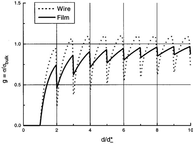
FIG. 2. Conductivities of semiballistic devices with very low disorder, in the second order Born approximation. The solid line represents the conductivity of a disordered film of width  $d$  as it goes through multiples of the resonant width  $d^*$ . The dashed line gives the conductivity of a 1D constriction of a 2D electron gas as a function of the width  $d$ .
