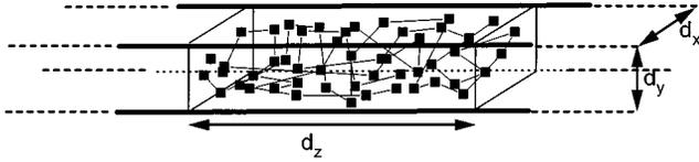
FIG. 1. The waveguide (with cross section  $d_x d_y$ ) is infinitely long, but the disorder is only present in a finite section of length  $d_z$ . The infinitely long pure sections act as ideal quantum leads.
