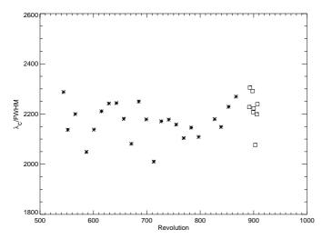
**Fig. 4.** Spectral resolution from the line-widths observed on the H Pfund  $\delta$  line [3.297  $\mu$ m] in NGC 6543. Asterisks are the values during the nominal mission. the squares are the values measured during the post-He phase. The lines were scanned using the AOT2 observation mode or an equivalent engineering mode after helium boil-off.
