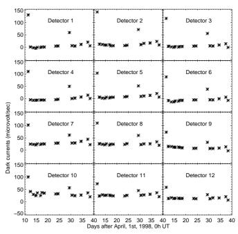
**Fig. 5.** The variation of the mean detector dark signals during the posthelium phase.
