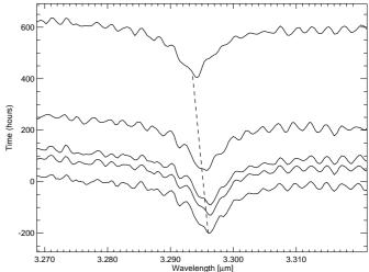
**Fig. 3.** As temperatures changed, geometry changes in the grating scanner mechanism induced a shift in the position of spectral features. We see the hydrogen Pfund Beta line in the spectrum of Alpha Lyrae. The time between the measurements was used to offset the different spectra in the figure.
