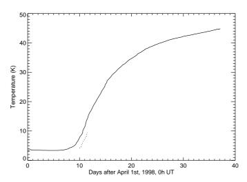
**Fig. 2.** The temperatures of the optical support structure (lower short curve, dashes) and of the upper baffle of the ISO telescope (upper curve, solid line) increased smoothly during the post-He phase.
