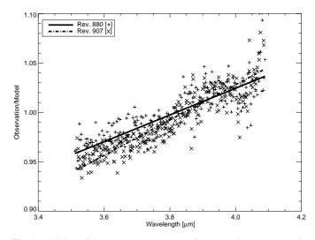
**Fig. 6.** Division of the observed spectrum of  $\gamma$  Draconis by a synthetic spectrum in the beginning and the end of the post-helium phase. The Relative Spectral Response of the SWS tilts more as the temperature increases.
