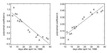
**Fig. 7.** Characterisation of the changing slope of the RSRF for detector 7 in AOT-band 1A. The triangles are the polynomial coefficients of the fits to the slope difference between calibration observations and model spectra. The solid line is a linear fit to the coefficients against time.
