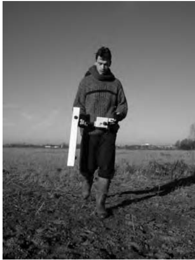
Figure 13 A Geoscan fluxgate gradiometer with 0.5 meter sensor separation (left) and a Bartington fluxgate gradiometer with 1 meter sensor separation (right).
