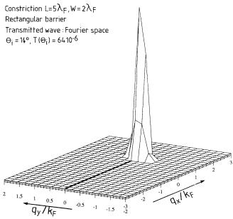
FIG. 4. Fourier transform of the wave packet emitted by a constriction followed by a rectangular barrier. TDSE simulation
