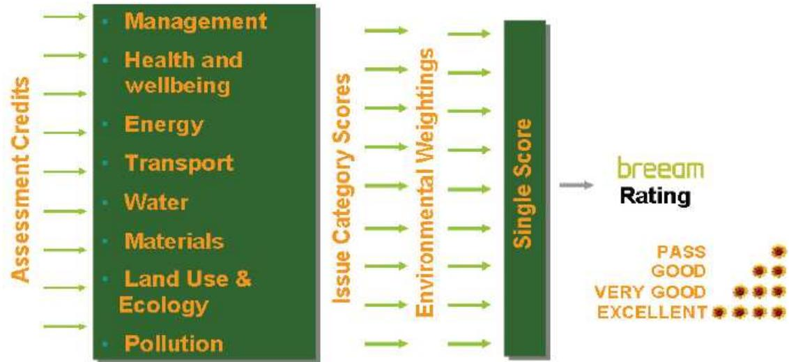
**Figure 1: BREEAM certification process** (Source: BRE, 2007).
