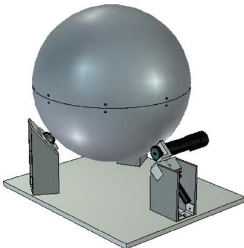
**Fig. 1** Ball RPM. The ball RPM is supported on two freely rotating contact points. The third contact point is a wheel connected to a motor that drives the rotation of the large sphere. The orientation of this motor and drive wheel can be varied by a second motor. The combined control of these motors allows a free walk path over the sphere, resulting in a continuously change in orientation of the sphere with its suspended sample system
