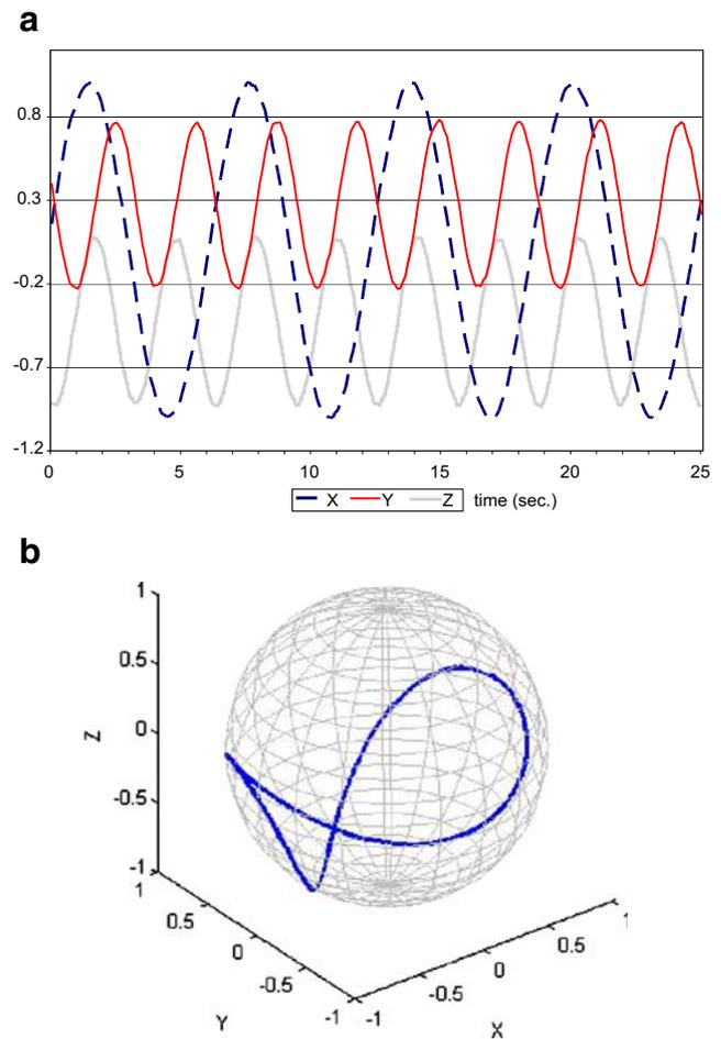
**Fig. 4** **a** Gravity values measured on the RPM, rotated in 3D clinostat mode, the inner and outer frame rotate (in this example) both at a constant speed of 60°/s. **b** Motion trajectory 3D clinostat mode with constant speed for both frames of 60°/s, displayed on an imaginary sphere. The abscissa in **a** as well as the three axes in **b** are accelerations expressed as ‘g’. Time displayed in seconds is displayed at the ordinate in **b**
