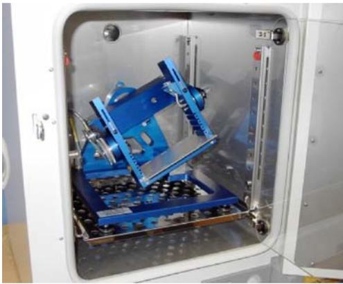
**Fig. 7** Desktop RPM in a standard incubator
