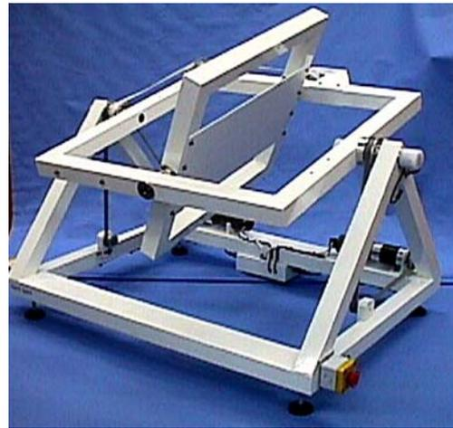
**Fig. 2** RPM with two independently driven perpendicular frames
