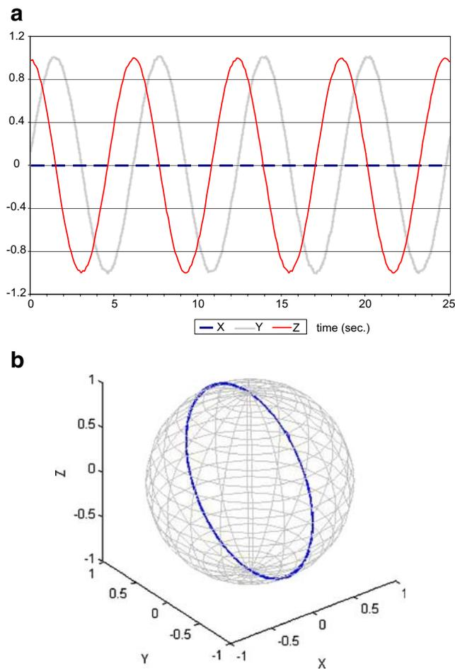
**Fig. 3** **a** Gravity values in a standard clinostat mode. Y and Z are changing sinusoidal between +1 g and -1 g. **b** The clinostat mode results in a 2D motion trajectory, in this graph projected on an imaginary sphere. The abscissa in **a** as well as the three axes in **b** are accelerations expressed as ‘g’. Time displayed in seconds is displayed at the ordinate in **b**
