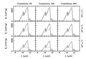
**Fig. 4.** The effective mass absorption coefficient of the crystalline forsterite component in the aggregates (full lines). The plots are organized as in Fig. 2. As a reference we also plot the mass absorption coefficients for an aggregate with the same size but composed of pure crystalline forsterite (dashed line).
