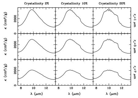
**Fig. 2.** The total mass aborption coefficients for the aggregates with crystalline silicate fraction (forsterite + enstatite) of 2% (*left panels*), 10% (*middle panels*), and 20% (*right panels*). The volume equivalent radii of the aggregates are 1  $\mu$ m (*upper panels*), 3  $\mu$ m (*middle panels*), and 7  $\mu$ m (*lower panels*).
