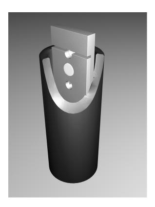
**Figure 6.2** Schematical representation of the test fixture. The two-plate specimen assembly fits precisely in the diametrically opposed grooves. Therefore movement of the jig was only possible in one direction, ensuring a pure shear force.
