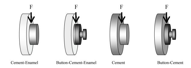
**Figure 6.1** Schematically representation of the four different specimens tested. The arrows indicate the location of force application during testing.
