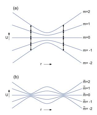
Figure 2.2: Comparison of the bare spin states in a static magnetic trapping potential for an atom with F=2 (a) and the states in an rf-dressed potential (b). The static magnetic field is that of a waveguide [Eq. (2.12) with  $r=\sqrt{y^2+z^2}$ ]. Plotted is the potential U against the spatial coordinate r. The arrows in (a) indicate the position where the rf is resonant with the energy spacing between the levels.
