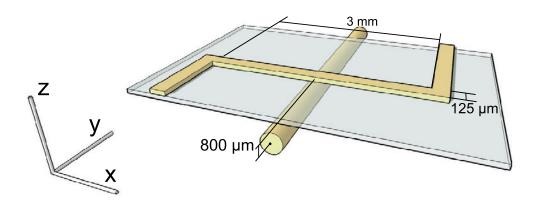
**Figure 2.1:** Geometry of the two most important field-generating wires in our magnetic trap. Dimensions of the wires are not to scale. The upper wire has a rectangular cross section and lies on a substrate. It has a Z-like shape. The wire underneath the substrate has a circular cross section. The coordinate system is also indicated.
