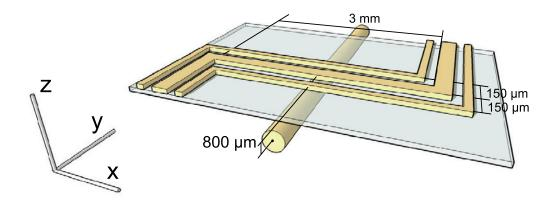
**Figure 2.3:** Sketch of both wires producing the static magnetic trap and the rf wires. The rf wires are positioned symmetrically with respect to the central Z wire. See Fig. 2.1 for the geometry without the rf wires.
