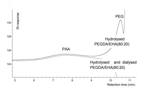
Fig. 2.5. Influence dialysis. SEC-RI chromatogram of hydrolysed PEGDA/EHA (80:20), before and after dialysis. Conditions as in Fig. 2.3.
