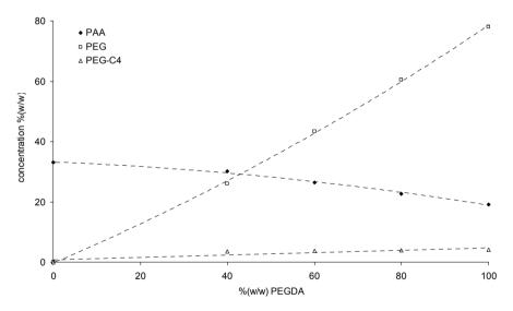
Fig. 2.8. Total concentration of PEG, PEG-C<sub>4</sub> and PAA in UV-cured PEGDA/EHA networks obtained by hydrolysis SEC-LC-RI-ESI(+)-MS, against PEGDA concentration.
