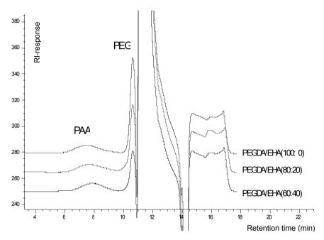
Fig. 2.3. SEC-chromatograms of hydrolysed UV-cured PEGDA/EHA polymers using RI-detection;  $8\times300$  mm Suprema column (PSS), 1000 Å, 10  $\mu$ m, flow= 1.0 mL/min 0.1 M NH<sub>4</sub>Ac, T=25°C,  $V_{inj}$ =20  $\mu$ L.
