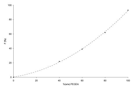
Fig. 2.12. Average degree of cross-linking of the PAA units as calculated by formula 2.1 and 2.2.
