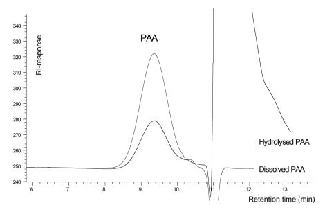
Fig. 2.4. SEC-chromatogram of dissolved and hydrolysed polyacrylic acid ( $M_{\rm w}$  2 kDa) using RI-detection. Conditions as in Fig. 2.3.
