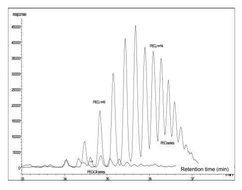
Fig. 2.6. Mass-reconstructed chromatogram of PEG and PEG- $C_4$  of a hydrolysed PEGDA/EHA(60:40) sample analysed by SEC-LC. Conditions; 8×300 mm Suprema 1000 Å coupled to 250×4.6 mm ODS-3 column, 1.0 mL/min, 20  $\mu$ L, RT, gradient; 0–10 min, 100% 0.1 M NH<sub>4</sub>Ac, 10–30 min from 0–50% acetonitrile, where it remains constant for 30 min.
