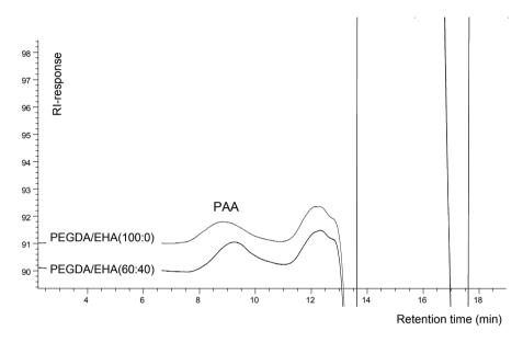
Fig. 2.7. SEC-LC-RI chromatograms of hydrolysed UV-cured acrylates. Conditions as in Fig. 2.6.
