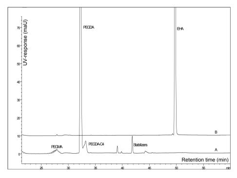
Fig. 2.2. UV-chromatogram ( $\lambda$  = 210 nm) of PEGDA (A) and EHA (B). Conditions: 250×3 mm ODS-3, 0.5 mL/min, 40°C, 5  $\mu$ L, gradient; 0–5 min, 100% H<sub>2</sub>O, 5–45 min from 0–100% acetonitrile, where it remains constant for 15 min.
