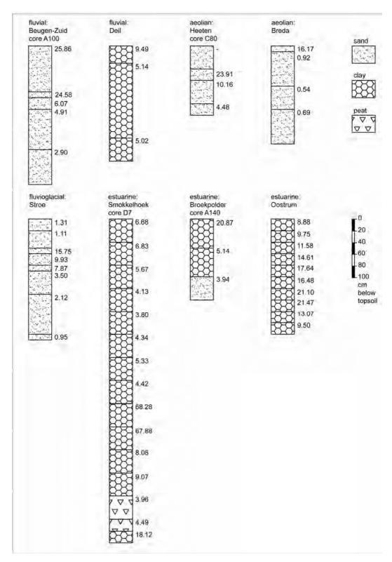
Figure 8 The magnetic susceptibility of eight typical soil profiles. Values on the right hand side of the cores represent the magnetic susceptibility x  $10^{-8}$  m $^3$ /kg. For matters of clarity the soil descriptions have been simplified to the three main classes of sand, clay and peat. Detailed soil descriptions of these profiles can be found in Appendix III.
