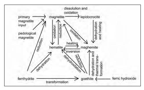
Figure 6 Schematic representation of a number of important transformation processes between the most common soil iron oxides in the Dutch soil.
