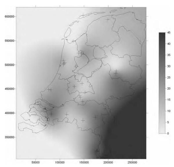
Figure 7 Topsoil magnetic susceptibility in The Netherlands from samples in this study, scale 8 x 10<sup>-8</sup> m<sup>3</sup>/kg. Crosses indicate the sample locations. Data has been gridded using the minimum curvature routine, which gives the smoothest possible surface and is more suitable for small and scattered datasets than other interpolation methods like for example Kriging.
